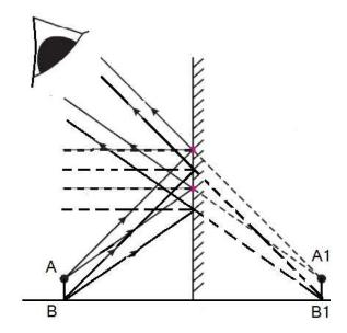
Draw two rays of light from a point to the mirror. Draw their reflected rays backwards. The point at which the reflected rays meet gives the image.
