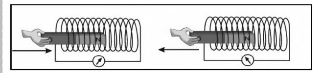
Electric current is produced in the circuit when an experiment is setup as shown in figure.
