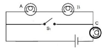
A, B and C are bulbs of the same power. Which bulbs will glow when S<sub>1</sub> is switched on?
