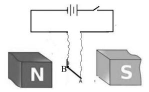
A conductor AB is placed in a magnetic field such a way that it can move freely.
