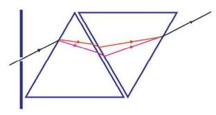
Place another inverted prism close to the first prism in the path of the dispersed light from a prism. The second prism must be similar to the first one. In the second prism those with higher wavelength reach near the base and those with lower wavelengths near them. In the first prism the colours get separated according to their wavelengths. In the second prism they get recombined.
